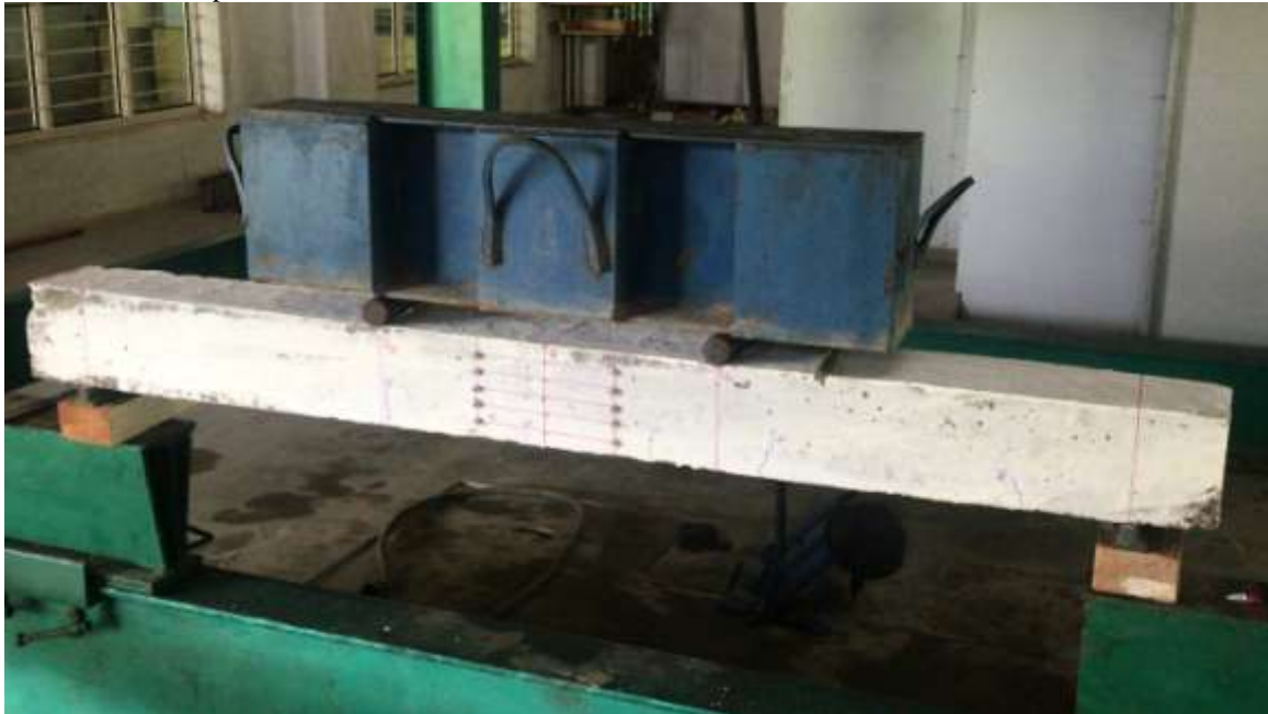
Fig ii4.3.1: iiTesting iiof iibeams iibefore iiretrofitting iand iininitial icracks iiare iimarked
