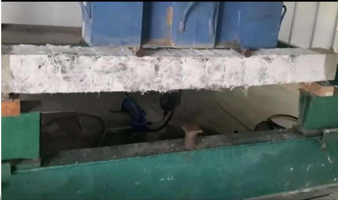
Fig ii3.4: iiCombination ii of ii45degree ii and ii90 ii degree ii strip ii wrapping ii using ii glass ii fiber ii sheetsii (white ii cement ii applied)
