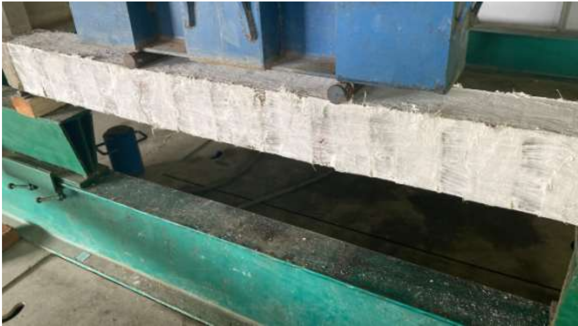
Fig ii4.4.1:90 iidegree iiwrapped iicollapsed iibeam iifor iiretrofitting
