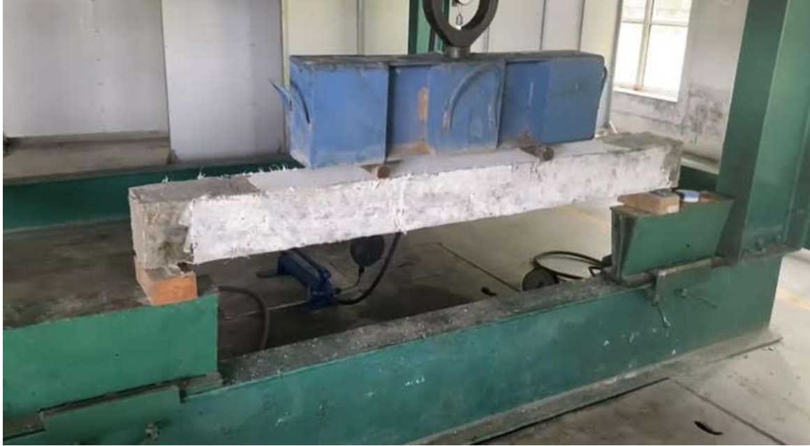
Fig ii4.4.3: iiU iiwrapped iicollapsed iibeam iifor iiretrofitting
