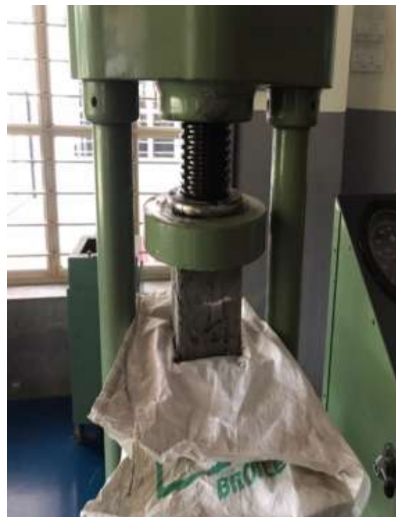
Fig 4.1.2: Compression test for cube specimen
