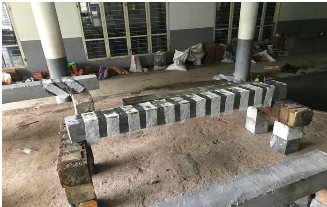
Fig ii3.3: ii90 iidegree iiwrapping iusing iiglass iifiber iisheets
