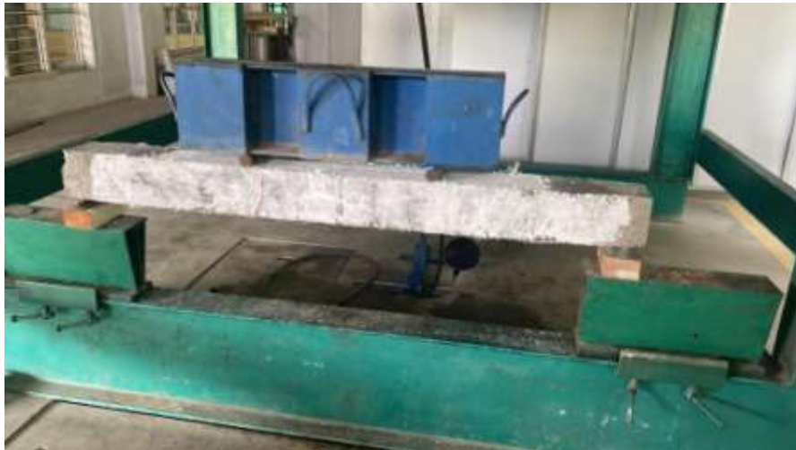
Fig ii4.3.3: iiTesting iiof iibeams iiafter iiretrofitting iiwith iiwrapped iiglass iifiber iisheets
