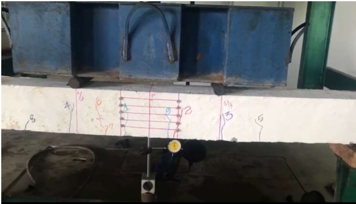
Fig ii4.3.2: iiCracked iispecimen iimarked ii
